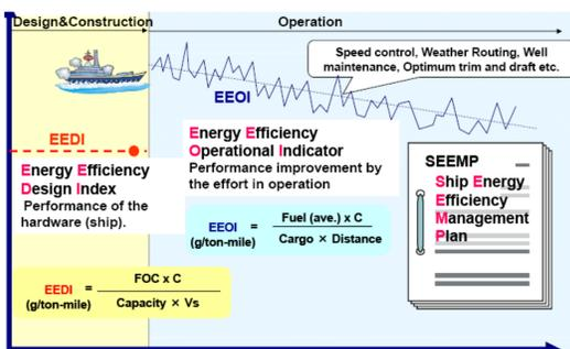
Energy efficiency regulations for ships covers both ship design and ship operation as shown in the above and below figures
